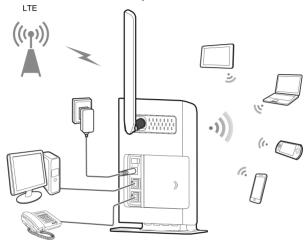
When the device is in use, you can alter its position or orientation to improve signal reception. The signal strength light indicates the received signal strength.
