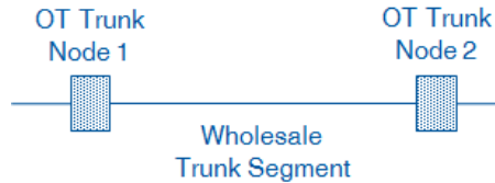
Figure 3-1 Trunk Segment of Leased Line
